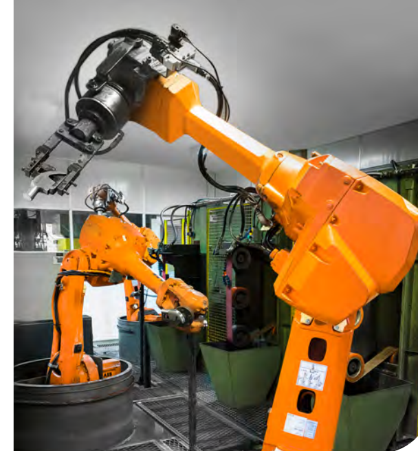
| Automated hammer grinding cell
